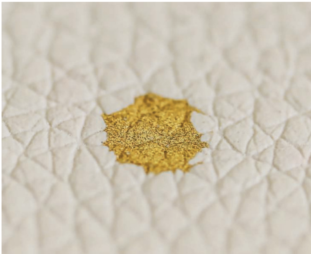
Flexible gold films can be transferred in a liquid droplet to coat irregular surfaces such as a model of human skin, seen here.
